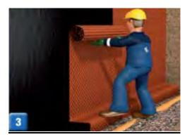
Placement of the HDPE egg casket, **PROTECDRAIN**, as a protection of the waterproofing layer from the impending embankment and as a drainage layer. **PROTECDRAIN** is mechanically bond above the waterproofing sealing with metal support. The earth backfill is recommended to be done step by step.
